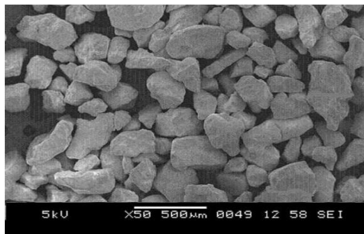
Figure 2(b): SEM Picture of Silica Sand (200-250 µm)
