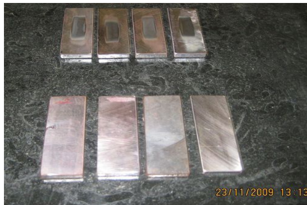
Figure 1: Standard test specimen (75x26x6 mm)
