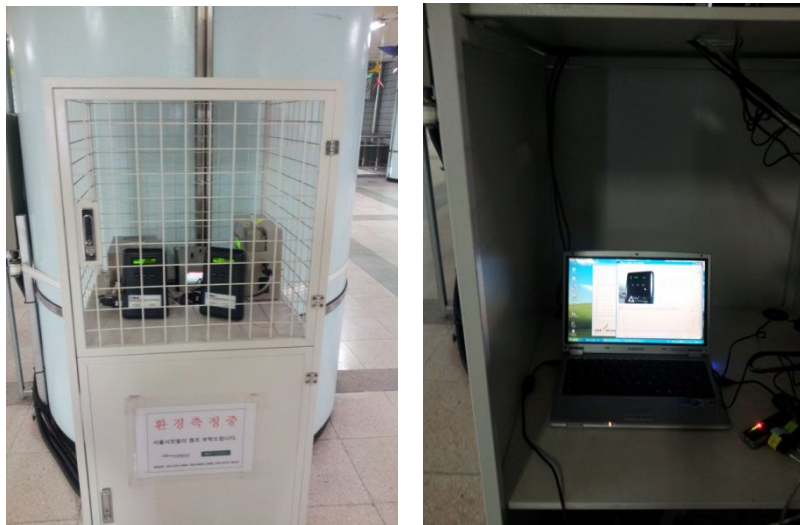
Fig. 1 PM measuring instruments in a subway station
