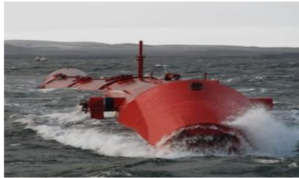
Fig. (2) This device looks like a sea snake in the water. It consists of a series of joints that generate power as the waves move them up and down through hydraulic rams and a generator. An underwater cable moves the electricity to the shore.
