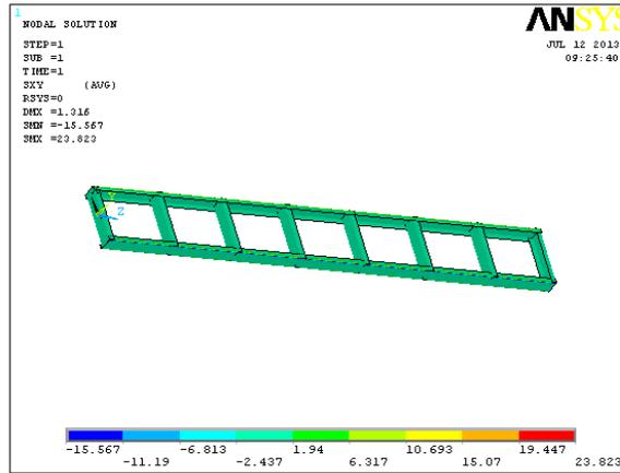
Fig. SHEAR STRESS IN XY
