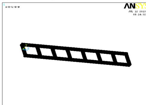
*Fig. Meshed Model Pressure – 0.06N/mm<sup>2</sup>*
