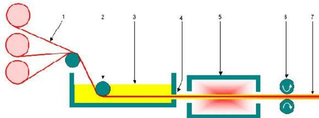
Fig: Pultrusion process steps
