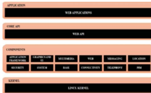
*Fig.2. Tizen architecture for smart phones and tablet devices.*
