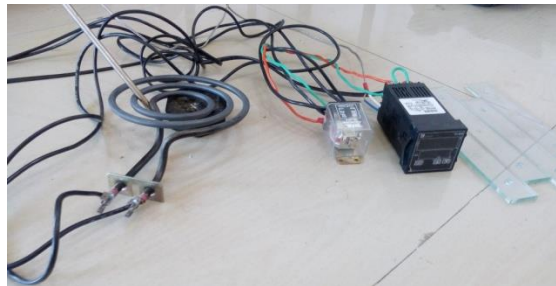
Fig .3 (Heating System)
