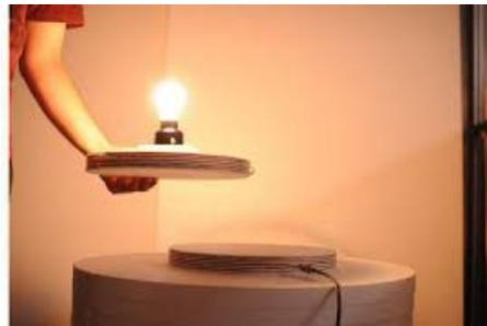
Researchers have developed several techniques for moving electricity over long distances without wires some exists only as theories or prototypes, but others are already in use. This paper provides the techniques used for wireless power transmission.
